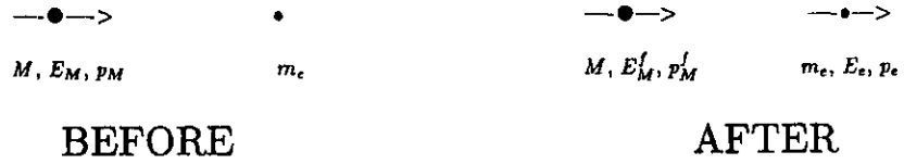
Fig. 3. A projectile of mass M , energy E_M and momentum p_M makes a head-on collision with an electron of mass m_e . In the final state, the energies and momenta are given by E_M^f, p_M^f , and E_e, p_e .
