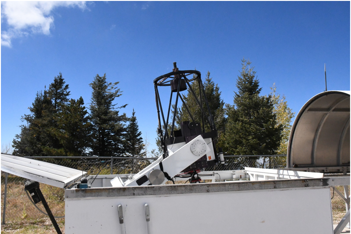
Figure 7: University of Louisville’s “Manner Telescope”, an 0.6-meter Ritchie-Chrétien located at the University of Arizona’s Stewart Observatory on Mt. Lemmon near Tucson.
